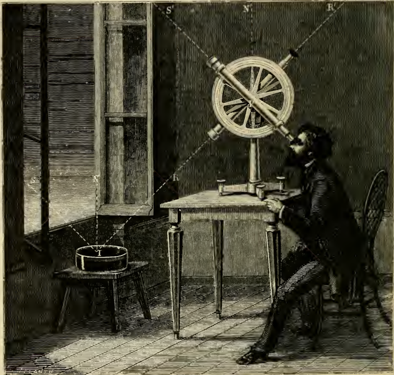
FIG. 48.—Experimental Proof that the Angle of Incidence = Angle of Reflection.
